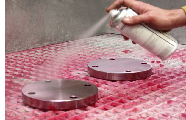
Dye Penetrant Test
